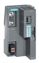
\*\*\* spare part \*\*\* SIMATIC DP, IM151-7 CPU for ET200S, 128 KB work memory with integrated PROFIBUS DP interface (9-pole D-sub socket) as DP Slave, without battery SIMATIC MMC required
