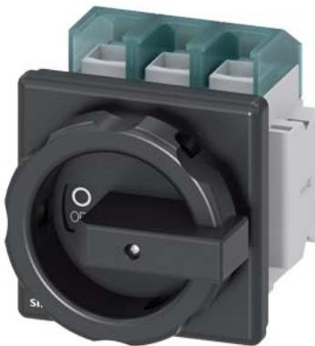
SENTRON, Switch disconnector 3LD, main switch, 3-pole, I<sub>u</sub>: 125 A, Operating power / at AC-23 A at 400 V: 45 kW, front-mounted, 1 NC, 1 NO, rotary operating mechanism, black, 4-hole mounting of the handle
