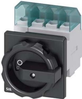
SENTRON, Switch disconnector 3LD, main switch, 4-pole, I<sub>u</sub>: 32 A, Operating power / at AC-23 A at 400 V: 11.5 kW, front-mounted, rotary operating mechanism, black, central mounting 22.5 mm of the handle
