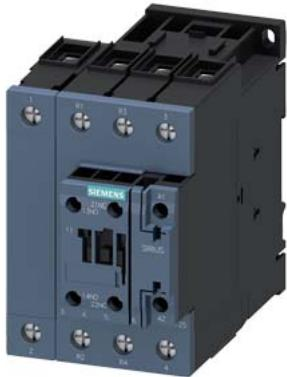
power contactor, AC-3, 35 A, 18.5 kW / 400 V, 4-pole, 83-155 V AC/DC, 50/60 Hz, with integrated varistor, main contacts: 2 NO + 2 NC, auxiliary contacts: 1 NO + 1 NC, screw terminal, size: S2
