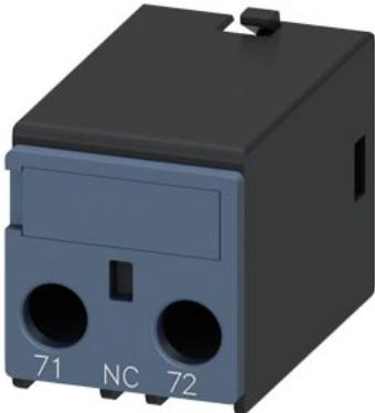
auxiliary switch, on the front, 1 NC, 71/72, current path: 1 NC, cable entry from below, screw terminal, for contactors 3RT2 and contactor relays 3RH2
