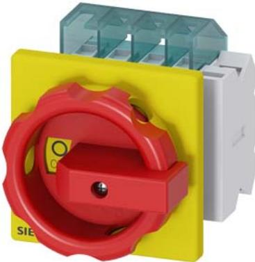
SENTRON, Switch disconnector 3LD, emergency switching-off switch, 3- pole, Iu: 16 A, operating power / at AC-23 A 400 V: 7.5 kW, front-mounted, 1 NC, 1 NO, rotary operating mechanism, Red / yellow, 4-hole mounting of the handle
