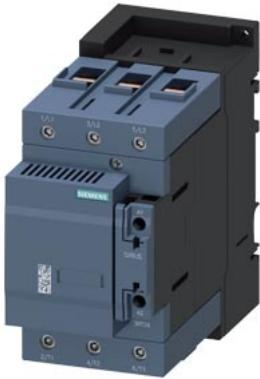
capacitor contactor, AC-6b 75 kVAr, / 400 V, 3-pole, 83-155 V AC/DC, 50/60 Hz, with integrated varistor, auxiliary contacts: 2 NC, screw terminal, size: S3
