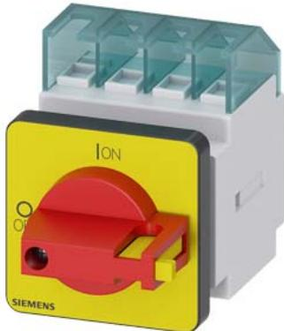
SENTRON, Switch disconnector 3LD, emergency switching-off switch, 3- pole, Iu: 16 A, operating power / at AC-23 A 400 V: 7.5 kW, front-mounted, knob-operated mechanism, red/yellow, 4-hole mounting of the handle
