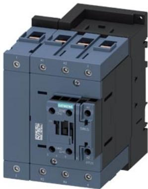
power contactor, AC-3, 65 A, 30 kW / 400 V, 4-pole, 20-33 V AC/DC, 50/60 Hz, with integrated varistor, main contacts: 2 NO + 2 NC, auxiliary contacts: 1 NO + 1 NC, screw terminal, size: S3
