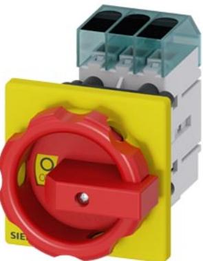
Load disconnector 3LD3, Iu 16 A Main switch 3-pole Rated operating capacity at AC-23 A at 400V 7.5kW Front plate mounting Basic switch with Central hole mounting 22.5mm Rotary actuator red / yellow 66 x 66 mm
