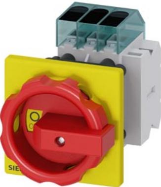
Load disconnector 3LD3, Iu 40 A Main switch 3-pole Rated operating capacity at AC-23 A at 400 V 18.5 kW Front plate mounting Basic switch with Central hole mounting 22.5mm Toggle drive red / yellow 66x66 mm with auxiliary switch 1OE + 1S
