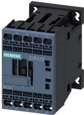
power contactor, AC-3, 9 A, 4 kW / 400 V, 4-pole, 24 V DC, main contacts: 2 NO + 2 NC, spring-loaded terminal, size: S00
