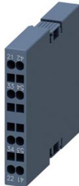
auxiliary switch, lateral, 1 NO + 1 NC, on the left: 41/42, 53/54, on the right: 21/22, 33/34, current path: 1 NC, 1 NO, spring-loaded terminal, for contactors 3RT2.1
