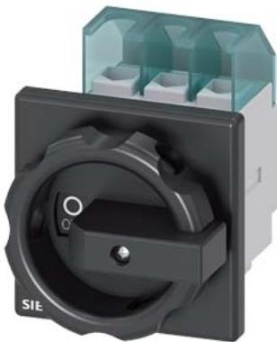
SENTRON, Switch disconnector 3LD, main switch, 3-pole, I<sub>u</sub>: 25 A, Operating power / at AC-23 A at 400 V: 9.5 kW, front-mounted, rotary operating mechanism, black, 4-hole mounting of the handle
