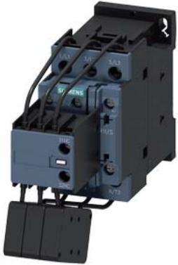
capacitor contactor, AC-6b 25 kVAr, / 400 V, 3-pole, 230 V AC, 50 Hz, auxiliary contacts: 1 NO + 2 NC, screw terminal, size: S0
