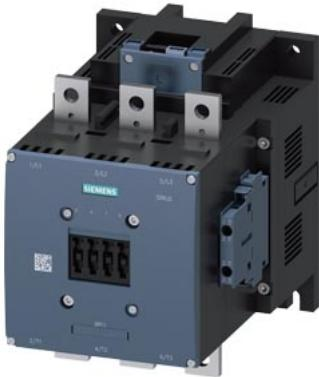
power contactor, AC-3e/AC-3 400 A, 200 kW / 400 V AC (50-60 Hz) / DC Uc: 21-27, 3 V PLC input 24 V DC 3-pole, auxiliary contacts 2 NO + 2 NC drive: electronic main circuit: busbar control and auxiliary circuit: screw terminal
