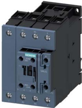
power contactor, AC-3, 35 A, 18.5 kW / 400 V, 4-pole, 110 V AC, 50 Hz / 120 V, 60 Hz, main contacts: 2 NO + 2 NC, auxiliary contacts: 1 NO + 1 NC, screw terminal, size: S2
