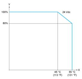
X: Ambient temperatureY: Input simultaneous ON ratio
