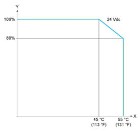
Ambient temperature Output simultaneous ON ratio
