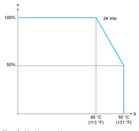
X: Ambient temperatureY: Input simultaneous ON ratio
