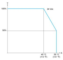
X : Ambient temperature Y : Output simultaneous Output simultaneous ON ratio
