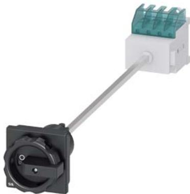
SENTRON, Switch disconnector 3LD, main switch, 3-pole, Iu: 16 A, Operating power / at AC-23 A at 400 V: 7.5 kW, floor mounting with door coupling, rotary operating mechanism, black, 4-hole mounting of the handle
