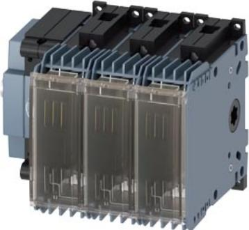
Switch disconnector with fuse 63 A, Size 1, 3-pole for LV HRC fuse Sz. 000 Side operating mechanism left Basic unit without handle Box terminal
