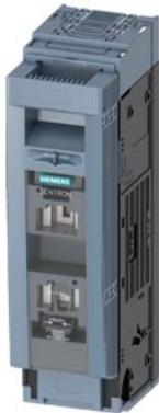
SENTRON, fuse switch disconnector 3NP1, 1-pole, NH2, 400 A, for assembly and installation on mounting plate, Flat terminal, cover level 70mm
