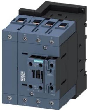
power contactor, AC-3, 80 A, 37 kW / 400 V, 4-pole, 24 V AC, 50 Hz, main contacts: 2 NO + 2 NC, auxiliary contacts: 1 NO + 1 NC, screw terminal, size: S3
