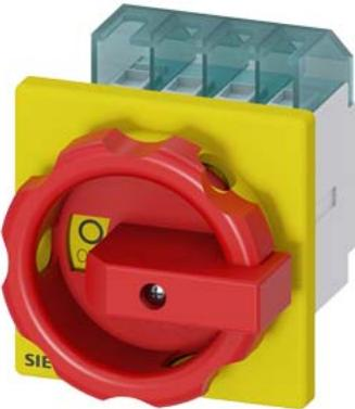
SENTRON, Switch disconnector 3LD, emergency switching-off switch, 4- pole, Iu: 16 A, operating power / at AC-23 A 400 V: 7.5 kW, front-mounted, rotary operating mechanism, Red / yellow, 4-hole mounting of the handle
