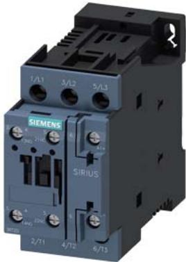
power contactor, AC-3e/AC-3, 12 A, 5.5 kW / 400 V, 3-pole, 24 V DC, auxiliary contacts: 1 NO + 1 NC, screw terminal, size: S0, communication-capable
