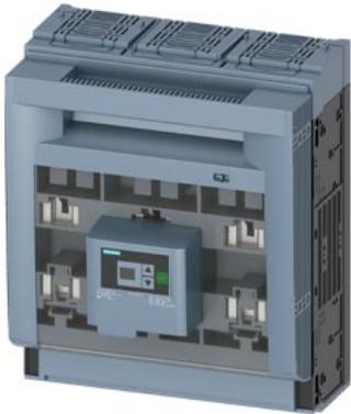
SENTRON, Fuse switch disconnector 3NP1, 3-pole, NH3, 630 A, for assembly and installation on mounting plate, flat terminal, Fuse monitoring: electronic EFM20, Cover level 70 mm
