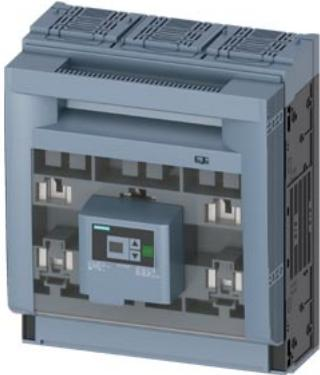
SENTRON, Fuse switch disconnector 3NP1, 3-pole, NH3, 630 A, for assembly and installation on mounting plate, Box terminal, Fuse monitoring: electronic EFM20, Cover level 70 mm
