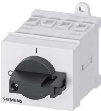
SENTRON, Switch disconnector 3LD, main switch, 3-pole, I<sub>u</sub>: 16 A, Operating power / at AC-23 A at 400 V: 7.5 kW, installation in distribution boards, knob-operated mechanism, black, handle direct at the switch
