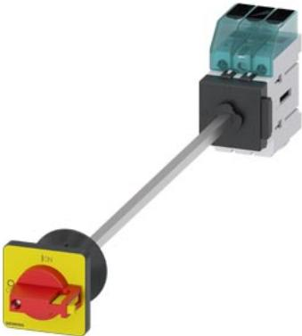
Load disconnector 3LD3, I<sub>u</sub> 40 A Main switch 3-pole Rated operating capacity at AC-23 A at 400 V 18.5 kW floor mounting Basic switch with door coupling Central hole mounting 22.5mm Toggle drive red / yellow 48x48 mm
