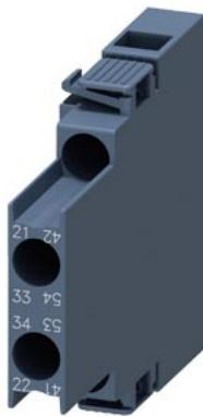
auxiliary switch, lateral, 1 NO + 1 NC, on the left: 41/42, 53/54, on the right: 21/22, 33/34, current path: 1 NC, 1 NO, screw terminal, for contactors 3RT2.1
