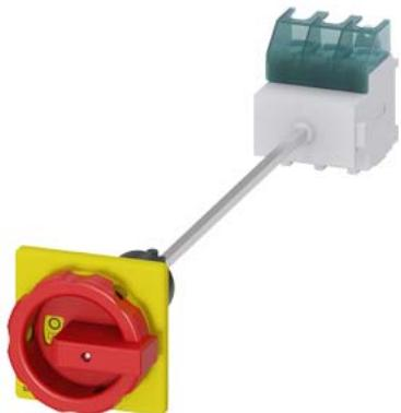
SENTRON, Switch disconnector 3LD, emergency switching-off switch, 3- pole, Iu: 63 A, operating power / at AC-23 A 400 V: 22 kW, floor mounting with door coupling, rotary operating mechanism, Red / yellow, central mounting 22.5 mm of the handle
