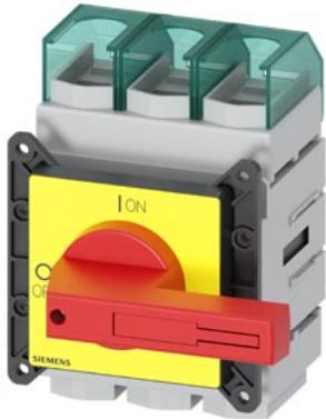
SENTRON, Switch disconnector 3LD, emergency switching-off switch, 3- pole, I<sub>u</sub>: 160 A, operating power / at AC-23 A 400 V: 75 kW, front-mounted, knob-operated mechanism, red/yellow, 4-hole mounting of the handle
