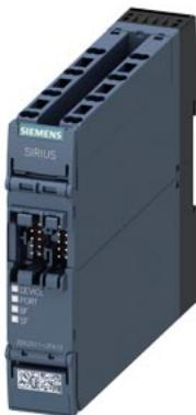
SIRIUS, interface module PROFINET interface for safety relay 3SK2 as of E05 and 3RK31 as of E04 PROFINET IO interface 100 Mbit/s, RJ45 22.5 mm width Spring-type terminal Can be parameterized via Safety ES without connecting cable
