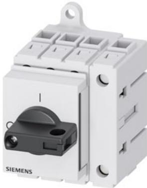
Load disconnector 3LD3, I<sub>u</sub> 25 A Main switch 3-pole + N Rated operating capacity at AC-23 A at 400V 9.0kW Installation in distribution boards, Basic switch with selector knob black
