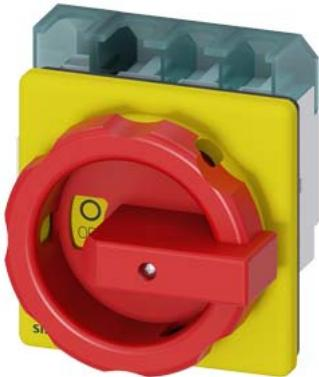
SENTRON, Switch disconnector 3LD, emergency switching-off switch, 4- pole, Iu: 63 A, operating power / at AC-23 A 400 V: 22 kW, front-mounted, rotary operating mechanism, Red / yellow, 4-hole mounting of the handle
