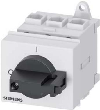
SENTRON, Switch disconnector 3LD, main switch, 3-pole, I<sub>u</sub>: 32 A, Operating power / at AC-23 A at 400 V: 11.5 kW, installation in distribution boards, knob-operated mechanism, black, handle direct at the switch
