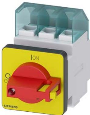
SENTRON, Switch disconnector 3LD, emergency switching-off switch, 3- pole, Iu: 25 A, operating power / at AC-23 A 400 V: 9.5 kW, floor mounting with door coupling, knob-operated mechanism, red/yellow, 4-hole mounting of the handle
