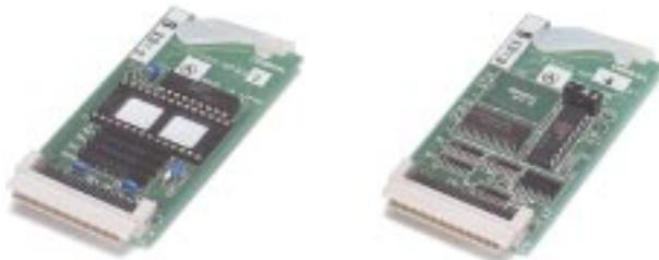
Choose either the EEPROM or the EPROM Memory Cassette to enhance the CQM1's memory. They will prevent the CQM1's Program Memory and DM from being lost during power interruption. The program and data in DM can be transferred between the CPU unit's RAM and the Memory Cassette. Data cannot be written to EPROM from the CPU unit.
