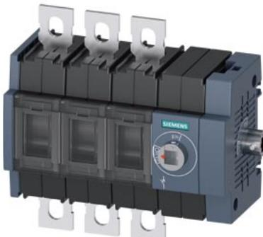
Switch disconnector 160 A, Size 2, 3-pole Lateral operating mechanism right Basic unit without handle flat terminal incl. phase barriers
