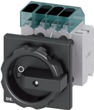
Load disconnector 3LD3, Iu 25 A Main switch 3-pole + N Rated operating capacity at AC-23 A at 400V 9.0kW Front plate mounting Basic switch with Central hole mounting 22.5mm Toggle drive black 66x66 mm with auxiliary switch 1OE + 1S
