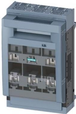
SENTRON, Fuse switch disconnector 3NP1, 3-pole, NH1, 250 A, for Rittal busbar system 60 mm, Box terminal, Cover level 32/70 mm
