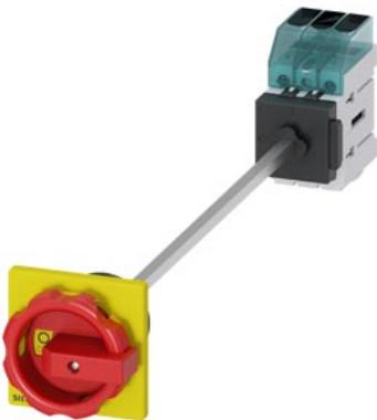
Load disconnector 3LD3, Iu 40 A Main switch 3-pole Rated operating capacity at AC-23 A at 400 V 18.5 kW floor mounting Basic switch with door coupling Central hole mounting 22.5mm Rotary actuator red / yellow 66 x 66 mm
