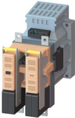
Contactor, size 12, 2-pole, DC-3 and 5, 400 A Auxiliary switch 22 (2 NO + 2 NC)
