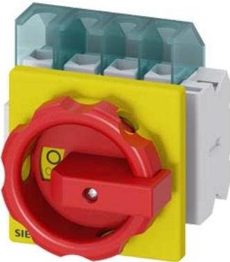
SENTRON, Switch disconnector 3LD, emergency switching-off switch, 4- pole, Iu: 25 A, operating power / at AC-23 A 400 V: 9.5 kW, front-mounted, 1 NC, 1 NO, rotary operating mechanism, Red / yellow, 4-hole mounting of the handle
