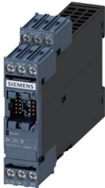
Digital module, 4 inputs and 2 relay outputs, input voltage 24 V DC, relay outputs bistable, max. 2 digital modules, for SIMOCODE pro V basic unit
