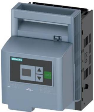
SENTRON, Fuse switch disconnector 3NP1, 3-pole, NH000, 160 A, for assembly and installation on Mounting plate, box terminal, Fuse monitoring: electronic EFM20, Cover level 45 mm
