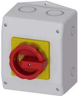
SENTRON, Switch disconnector 3LD, emergency switching-off switch, 6- pole, Iu: 32 A, operating power / at AC-23 A 400 V: 11.5 kW, molded-plastic encapsulation for metric screw connection, 1 NC, 1 NO, rotary operating mechanism, red/yellow
