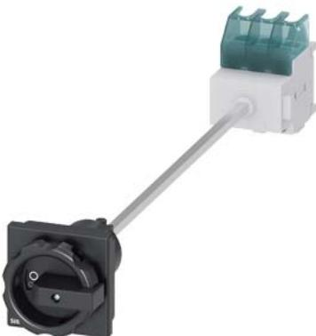
SENTRON, Switch disconnector 3LD, main switch, 3-pole, I<sub>u</sub>: 25 A, Operating power / at AC-23 A at 400 V: 9.5 kW, floor mounting with door coupling, rotary operating mechanism, black, 4-hole mounting of the handle
