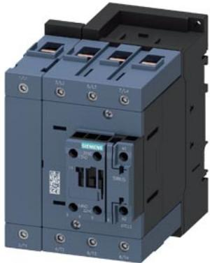
contactor AC-1, 160 A, 400 V / 40 °C, 4-pole, 20-33 V AC/DC, 50/60 Hz, with integrated varistor, auxiliary contacts: 1 NO + 1 NC, screw terminal, size: S3
