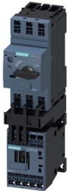
Load feeder fuseless, Direct-on-line starting 400 V AC, Size S00 2.80...4.00 A 230 V AC Spring-type terminal for installation on standard mounting rail (also fulfills type of coordination 1) Type of coordination 2,  $I_q = 150$  kA 1 NO (contactor)
