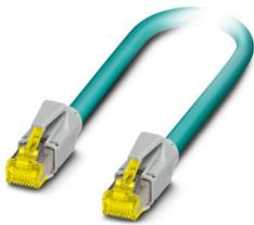
Patch cable, CAT6<sub>A</sub>, 4-pair, shielded, connection not crossed (line), assembled at both ends with RJ45/IP20 connectors, outer sheath material: PUR, length: 2.0 m
